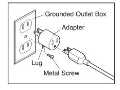
available. The temporary adapter should be used only until a properly grounded outlet can be installed by a qualified electrician.
